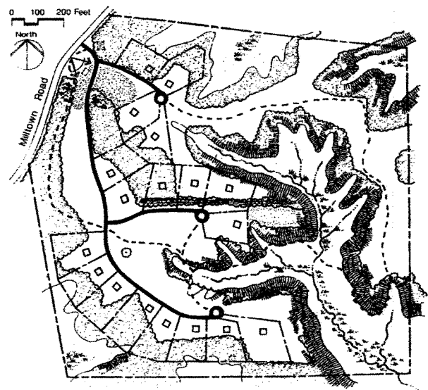
Figure 18 STEP FOUR Drawing in the Lot Lines
