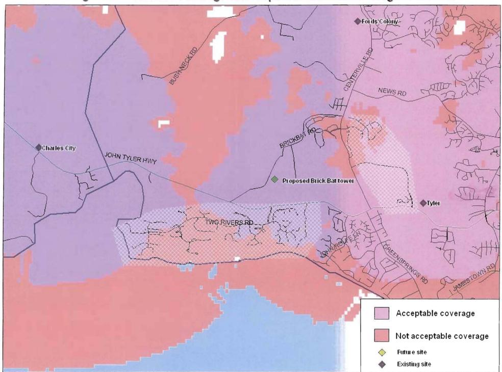
Existing Verizon Wireless Coverage with Proposed Brick Bat Coverage at 183 feet
