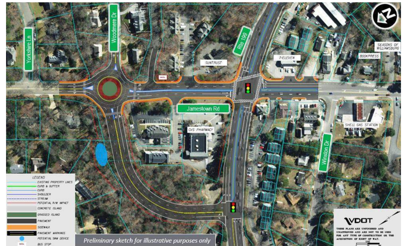
Figure 28: Phase 2 Alternative – Jamestown Road Quadrant with Roundabout
