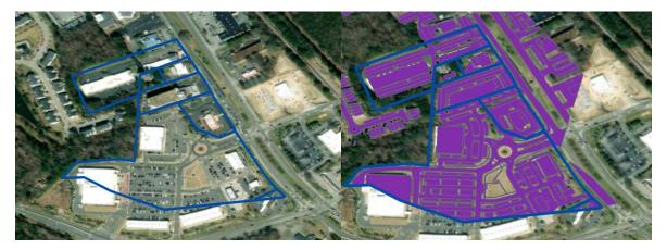
Figure 9 – Representative Commercial Sample, Existing Impervious Surface Area (Purple Area)
