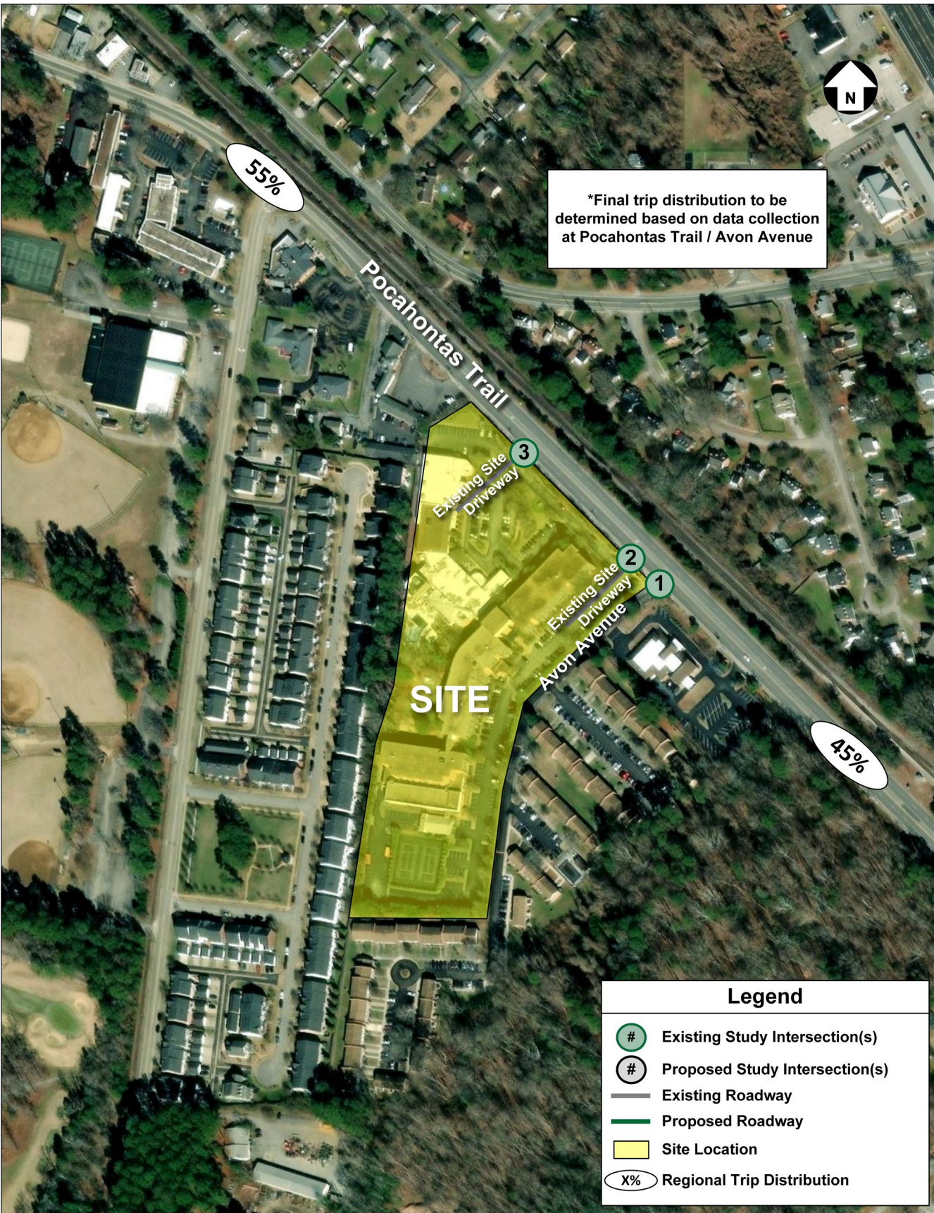
Figure 1: Study Intersections and Primary Site Trip Distribution
