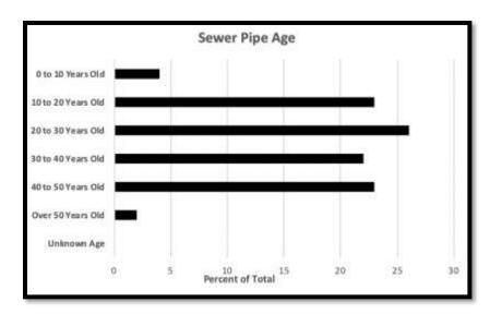
As the chart above shows, while the majority of JCSA pipe infrastructure is 10 to 30 years old, almost one quarter of the total is over 40 years old. In addition to material and age, other factors that can influence expected pipe life include soil type, installation and climate. The Repair and Replacement Reserve prepares JCSA to address challenges of aging infrastructure.
