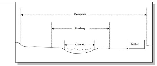
Floodway. The channel of a river or other watercourse and the adjacent land areas that must be reserved in order to discharge the base flood without cumulatively increasing the water surface elevation more than one foot.
