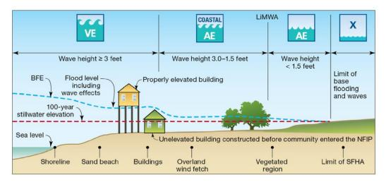
The area in front of the LiMWA line is also referred to as the "Coastal AE" zone. The "Coastal AE" zone is defined as areas that have been delineated as subject to wave heights between 1.5 feet and 3 feet and identified on the FIRM as AE areas that are seaward of the LiMWA line.
