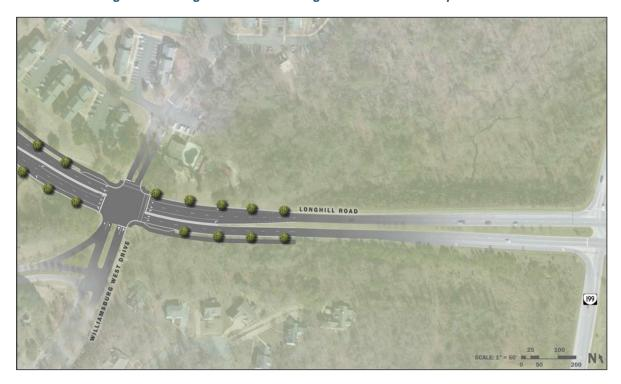
Figure 18: Longhill Road Widening and Intersection Improvements
