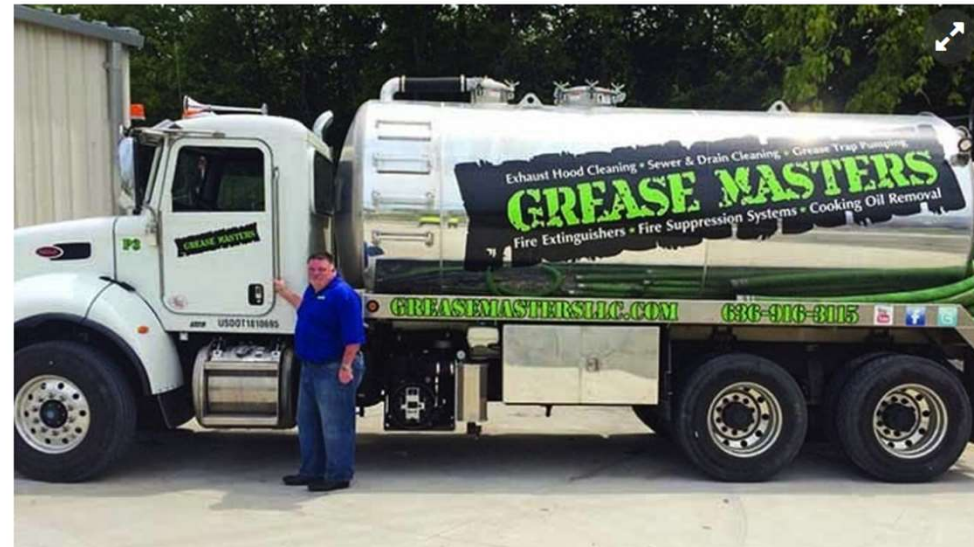
John Remstedt is shown with his newest truck, purchased at the WWETT Show. It's a 2015 Peterbilt built out by Satellite Industries and carrying a 4,000-gallon aluminum tank from Imperial Industries, a pump from National Vacuum Equipment Inc. (NVE) and a pressure jetter from Advance Pump & Equipment Inc., powered by a Giant pump. (Photo courtesy of Grease Masters)
