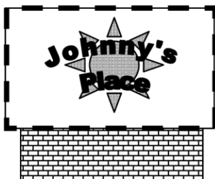
Figure 1c- Freestanding sign where letters/logos are mounted as a connected group
